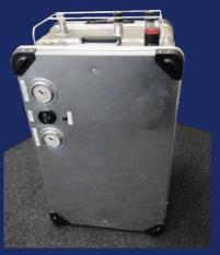
Furthermore, it has an emergency supply through 2 composite cylinders, which continue to supply the employees with breathing air in case of emergency. The cylinder storage system contains 4080 liters of breathing air in two 6.8 L / 300 bar composite cylinders. The breathing air is automatically used either from the operating air or from the reservoir. The air distribution works pneumatically and not electrically.
